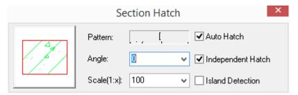
If we select options: "Independent Hatch" and "Island Detection", we do not have to close the region which is to be selected in advance, as GstarCAD Architecture will automatically find the closest closed region to fill in.
