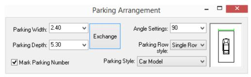
After we set the parking parameters in the dialog box, we can draw the rectangular parking consisting of Pline according to the interaction in the command line without closing the dialog box.
