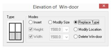
In the dialog box user can check the check box "Height" or "Width" and modify the parameter regarding one of them with that of the other unchanged, user can also check both of the two checkboxes and modify the parameters of them at the same time, then operate as per the prompt in the command line.
