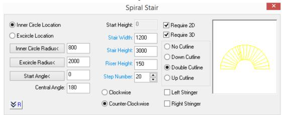
After entering the stair parameter in the dialog box, the user can determine whether the stair parameter entered can meet the requirement according to the dynamic preview window on the right of the dialog box. The options in the dialog box are similar to that of the straight stair. User can refer to the related description of the last section.
