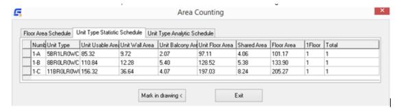
The third table "Unit Type Analytic Schedule" is rationally calculated by relation of room usable area and shared area. User can follow the same steps as the above to insert the table in the drawing.
