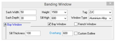
Sideboard is added to the right side of the corner bay window, and the "Overhang" is 600. After the execution of the command, the effect drawing is as shown in the right picture below.
