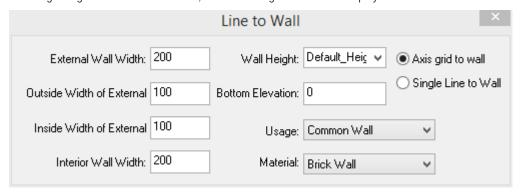
The radio box "Axis Grid to Wall" is clicked by default, at this time, only the axis grid layer and objects on it can be selected, and the command line prompts:
