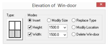
The function is similar to "Insert Elevation Win-Door" function. Click the image box on the left of the dialog box and select the elevation win-door required. Double click it to return back to the elevation win-door dialog box, and the command line will prompt:
