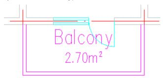
In GstarCAD Architecture, The area of the balcony is calculated as half of the actual area of it by default. User can decide whether to calculate it in this way by setting the related parameter in "Edit Room" dialog box.
