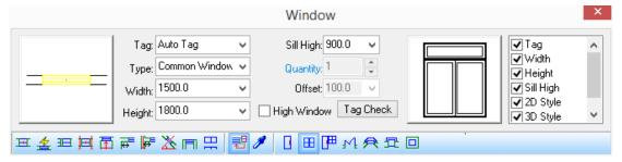
If user does not want to change some parameter during the replacing, please uncheck the related checkbox, after which, the parameter would remain unchanged and keep the same with that of the original drawing after the replacing. For example, if user does not want the width of the existing door to be changed when converting the door into a window, the "Width" check box should be unchecked.
