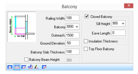
The tool bar at the bottom provides 6 methods to draw the balcony, there are "Concave Balcony", "Rectangle Triangle Balcony", "Internal Corner Balcony", "Offset Drawing along Wall", "Custom Draw", "Select Existed Path to Generate". After the check box "Balcony Beam Height:" is checked, user can enter the value for it to create balcony of beam type.
