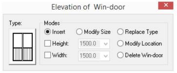
There are five main functions involved in the dialog box. They are: "Insert Elevation Win-Door", "Modify the Size of Elevation Win-Door", "Replace the Elevation Win-Door", "Modify the Location of The Elevation Win-Door" and "Delete the Elevation Win-Door". We will introduce these functions to you as follows:
