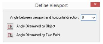
Enter proper parameter in the dialog box. Generally, the viewport will be arranged horizontally, in this case, the angle between viewport and horizontal direction would be 0. What we have to do is to enter the viewport output scale. If we want to define a sloping viewport, we can use any one of the three methods: "Specify Angle between Viewport and Horizontal Direction:", "Angle Determined by Object" and "Angle Determined by Two Point".
